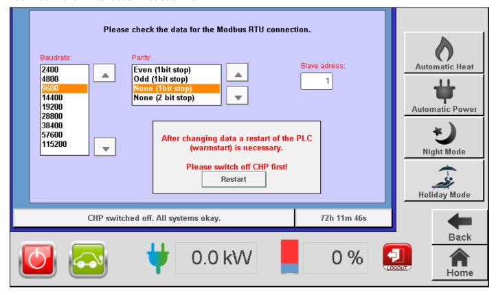
The following items can be set for connection via Modbus-RTU:
