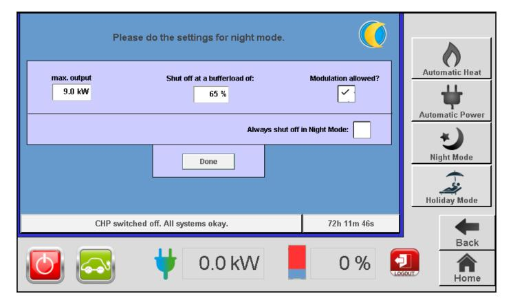
The following information is necessary, in order to specify the system behaviour in night operation:
