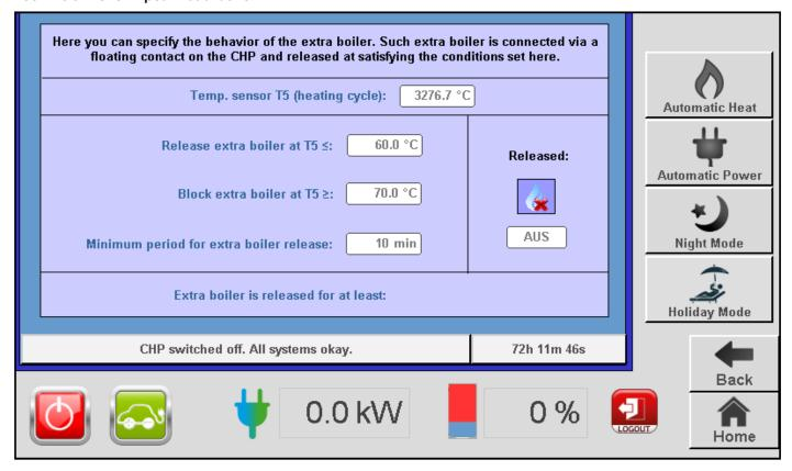
The system can control a connected peak load boiler via a potential-free contact (designed as an NC contact). Trained specialist personnel are able to stipulate the behaviour of the peak load boiler ("SLK") in this menu.
