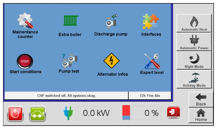
The logout symbol is displayed for access to the technician level. In order to log out of the technician level:
