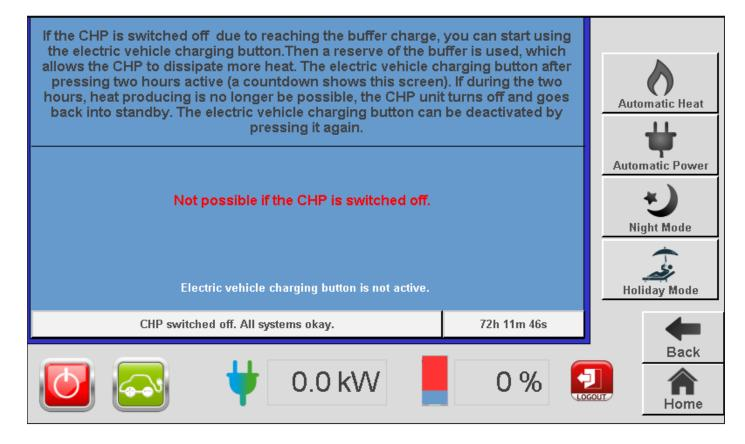
When the buffer tank is loaded, the system switches off. By touching the electric vehicle charging button it is possible to restart the system. This changes the regulation direction and a buffer reserve is used, so that the system can take off further heat.
