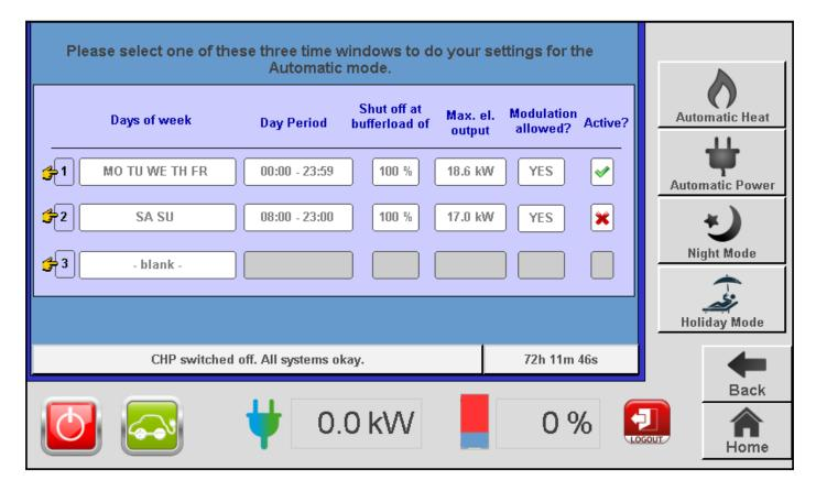
The runtime behaviour of the system is planned in the "Automatic mode settings" menu. Three time windows are available here.
