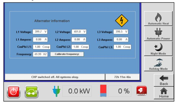
The following generator information is displayed for monitoring the generator output:
