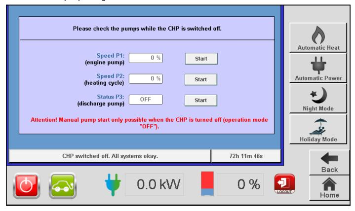
A pump test may be necessary after installation of the system, e.g. for flushing purposes. Trained specialist personnel are able to perform the pump test in this menu.
