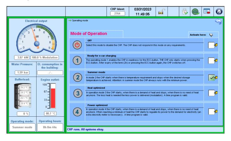
The system can be operated in five modes of operation (including shutdown).
