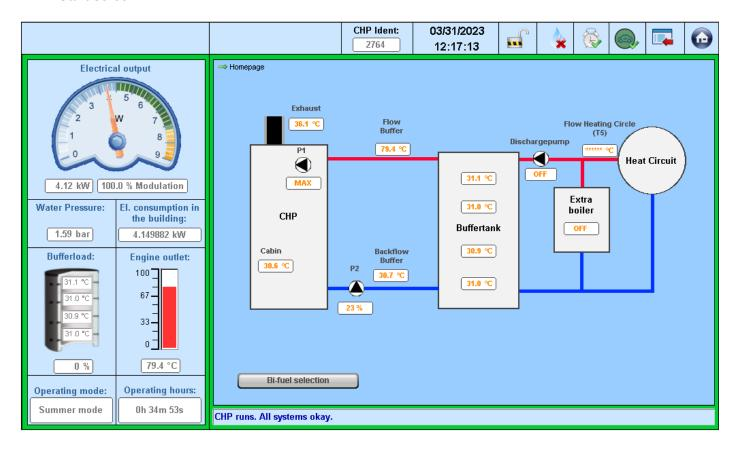
The start screen displays an overview of the actuated system in accordance with the hydraulic plan (the actual layout may vary).
