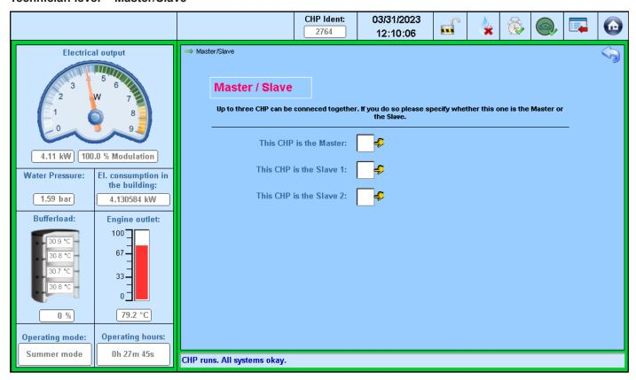
If two or more systems are installed then it is possible to connect the systems in a cascade. In cascade mode the participating systems are defined as "master" or "slave". The "master" performs the control for all connected systems. For example:
