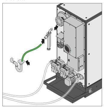
The line for the condensate water must be corrosion resistant.
