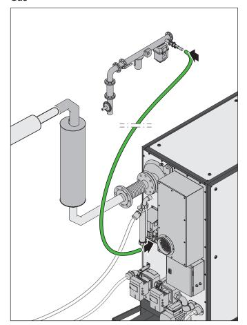
The gas supply must comply with the established regulations (e.g. in Germany, TRGI). Connection via a gas appliance outlet is not permitted.
