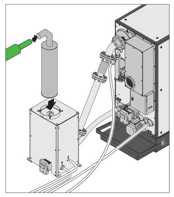
The line must be laid with a sufficient gradient to the calorific value heat exchanger.
