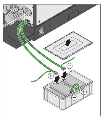
The batteries are located in the battery box.
